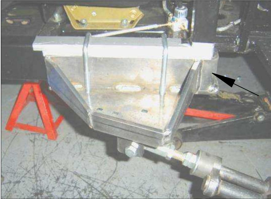
Put the L shape part against the structure's corner.
