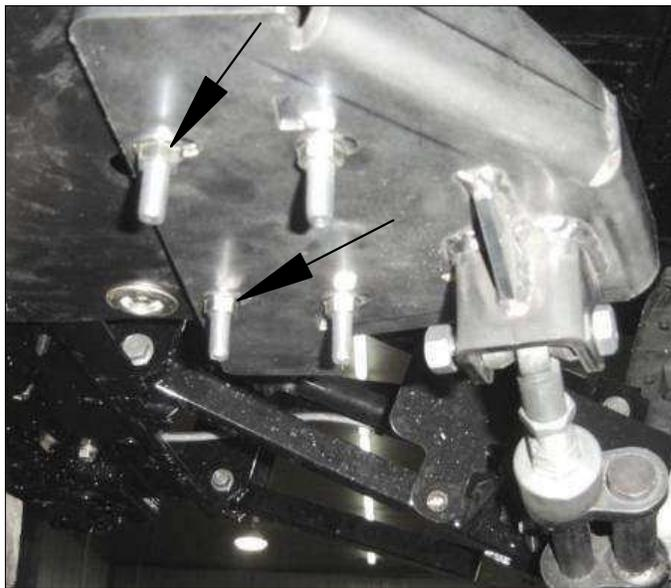
Attach well the plate 03PA-260G to the frame .
