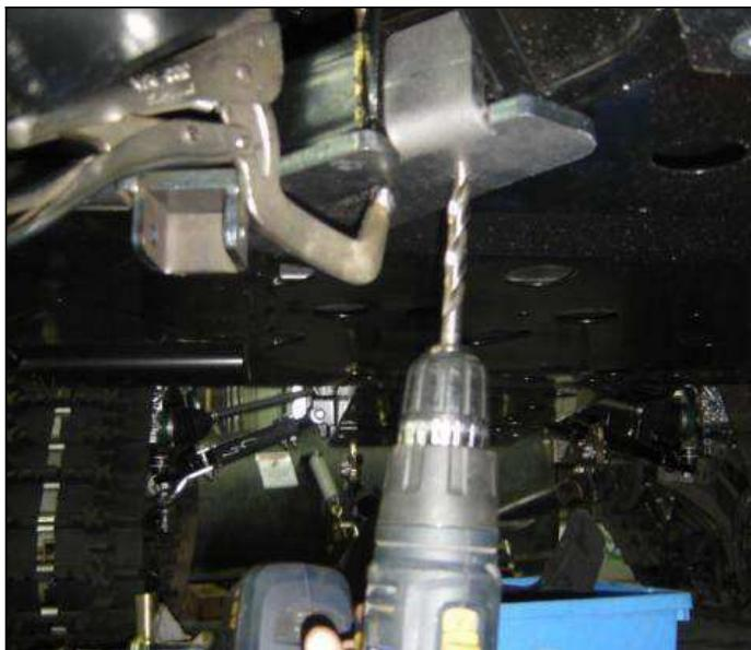
With a 13/32" drill, make holes in the atv's guard. Holes in the piece 03PA-261G will guide you.
