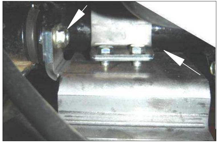
To install the part 03PA-268G and D you'll have to remove the nut that holds the front end of the leaf springs (left pic).
