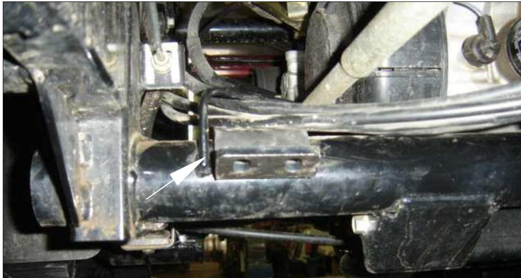
On the right side (passenger), you'll have to pass the part 04PL-169 underneath the U rod (see the arrow).
