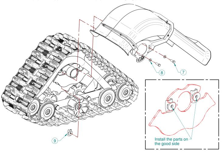
$\label{eq:STAGE-3} \textbf{STAGE-3} \textbf{ -} \textbf{ Adjust the fenders to have the same distance at the front and the rear.}$
