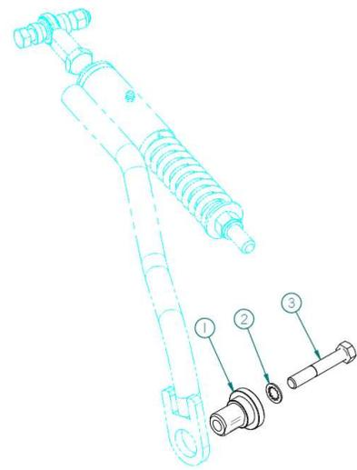
Remove the bolt and bushing spacers at the end of the rod. Then attach the stabilization rod to the adapter plate, making sure that the bushings are placed between the spacers and the rod support. If your stabilization rod support has three (3) positioning holes, use the central hole.
