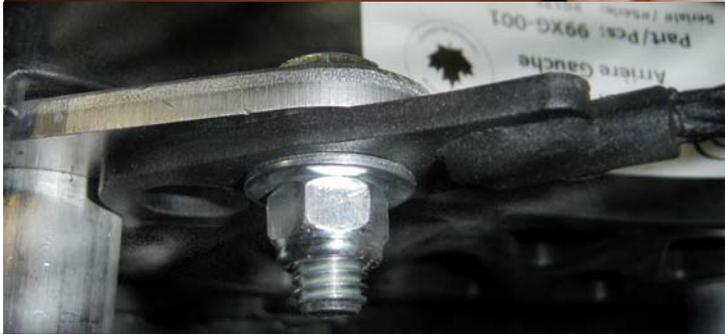
10. Remove the wooden bloc and tighten the track.
