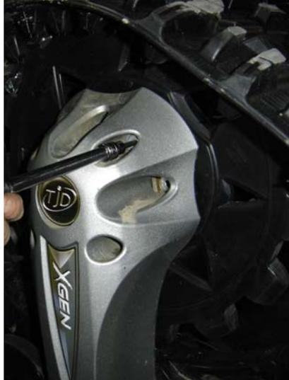
5. Space the sprocket from the suspension arm, 60mm approximately.
